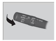
Disable or re-enable the system when the vehicle is parked and the power mode is in ON and the light switch is in the **AUTO** position. **Disabling the system:** Pull the light switch lever toward you and hold it for at least 40 seconds. The auto high-beam indicator in the meter will blink twice.
