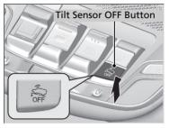
To turn off the tilt sensor system, press the tilt sensor OFF button after you set the power mode to ACCESSORY or VEHICLE OFF (LOCK). The is on in red.
