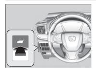
To open or close the power tailgate, press the power tailgate button for about one second. ► Some exterior lights will flash.
