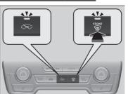
Pressing the real (windscreen demister) button turns the air conditioning system on and automatically switches the system to fresh air mode.
