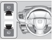
Turn the headlights on and press the headlight washer button to operate. The headlight washers also operate when you turn the windscreen washers for the first time after the power mode is in ON.
