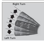
The turn signals can be used when the power system is in ON.
