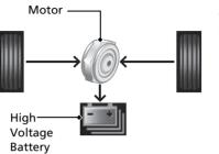
When decelerating without the accelerator being depressed or the brake pedal being applied, or while driving downhill, the electric motor acts as a generator that recovers a portion of the electrical energy that was used to accelerate the vehicle. This regenerative braking slows the vehicle in a manner similar to engine braking in a petrol-driven vehicle. You can control the rate of deceleration by using the deceleration paddle selector.
