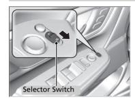
If activated, the passenger side door mirror automatically tilts downward when you put the transmission into  $[\mathbf{R}]$ ; this improves close-in visibility on the passenger side of the vehicle when backing up. The mirror automatically returns to its original position when you take the transmission out of  $[\mathbf{R}]$ .
