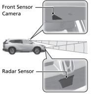
The radar sensor is in the front grille.
