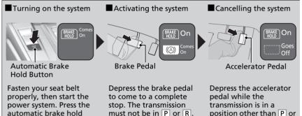
The automatic brake hold system indicator comes on. The system is turned on.
