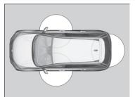
When you carry the keyless remote, you can lock/unlock the doors and open the tailgate. You can lock/unlock the doors and tailgate within a radius of about 80 cm of the outside door handle or tailgate outer handle.
