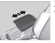
The console lid can be used as an armrest. **To adjust:** Slide the armrest to a desired position.
