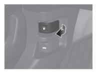
**2** Turn the fuel fill cap slowly to remove the cap.
