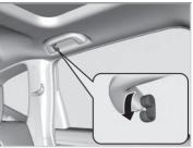
There are coat hooks on the rear left and right grab handles. Pull it down to use it.
