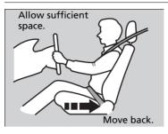
Adjust the driver's seat as far back as possible while allowing you to maintain full control of the vehicle. You should be able to sit upright, well back in the seat and be able to adequately press the pedals without leaning forward, and grip the steering wheel comfortably. The passenger's seat should be adjusted in a similar manner, so that it is as far back from the front airbag in the dashboard as possible.
