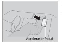
Gently depress the accelerator pedal. When on a hill, it may require more accelerator input to release.
