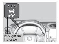
When VSA activates, you may notice that the engine and motor do not respond to the accelerator. You may also notice some noise from the hydraulic system. You will also see the indicator blink.
