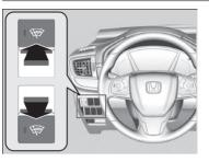
Press the heated windscreen button to deice the windscreen when the power mode is in ON.
