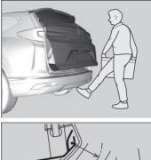
Use a forward and back kicking motion under the centre of the rear bumper to open or close the power tailgate while carrying the keyless remote.
