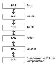
Rotate  $\ensuremath{\,\overline{\bigcirc}\,}$  to adjust the sound setting, then press  $\ensuremath{\,\overline{\bigcirc}\,}$  .
