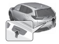
• Press the outer handle to unlock and open the tailgate when you have the keyless remote on you.
