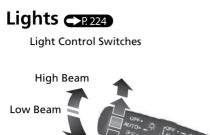
Flashing the high beams
