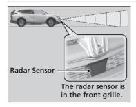
The radar sensor is in the front grille.
