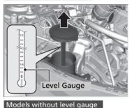
Check the amount of window washer fluid using the washer fluid level gauge on the cap.
