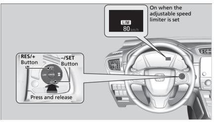
• Take your foot off the accelerator pedal and press the –/SET button when you reach the desired speed.
