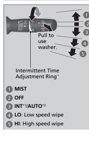
The windscreen wipers and washers can be used when the power mode is in ON.
