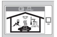
High temperature may damage the highvoltage battery used to power the electric motor.
