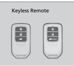
Use the keys to turn on and off the power system, and to lock and unlock all the doors and tailgate.
