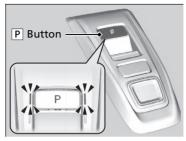
The shift position changes to  $\boxed{P}$  when you press the  $\boxed{P}$  button while the vehicle is parked with the power mode in ON. The indicators on the sides of the  $\boxed{P}$  button come on.
