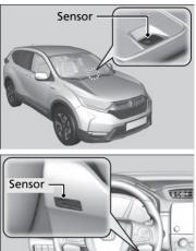
The automatic climate control system is equipped with sensors. Do not cover or spill any liquid on them.
