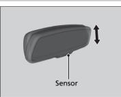
When you are driving after dark, the automatic dimming rearview mirror reduces the glare from headlights behind you, based in inputs from the mirror sensor. This feature is always active. Automatic Dimming Rearview Mirror\*
