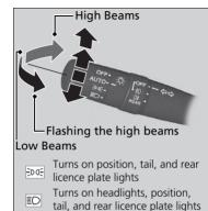
Rotating the light switch turns the lights on and off, regardless of the power mode setting.
