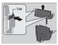
**4.** Pull out the fuse box inside the inner fender, then push the tabs to open the box.
