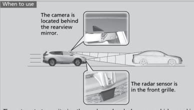
The system starts monitoring the roadway ahead when your vehicle speed is about 5 km/h (3 mph) and there is a vehicle in front of you.
