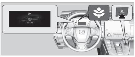
The **ECON** button turns the ECON mode on and off. The ECON mode helps you improve your fuel economy by adjusting the performance of the engine and climate control system.
