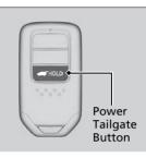
Press the power tailgate button for more than one second to operate when the power mode is in VEHICLE OFF (LOCK).
