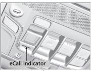
If your vehicle is involved in a collision, the SRS unit in the vehicle will attempt to connect to a Public Safety Answering Point (PSAP) operator. Once a connection is established, various information about the vehicle will be sent to a PSAP operator with whom you will be able to speak. This information includes:
