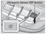
To turn off the ultrasonic sensor system, press the ultrasonic sensor OFF button after you set the power mode to ACCESSORY or VEHICLE OFF (LOCK).
