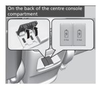
Install the iPod USB connector or the USB flash drive to the USB port.
