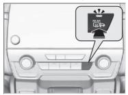
The rear demister and heated door mirror automatically switches off after 10-30 minutes depending on the outside temperature. However, if the outside temperature is 0°C or below, it does not automatically switch off.
