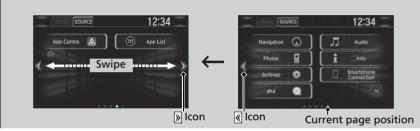
Selecting  $\overline{\langle\!\langle}$  or  $\overline{\rangle\!\rangle}$ , or swiping the screen left or right changes to the next screen.
