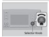
Press the **MENU/CLOCK** button and rotate or to select **Sound**, then press 3. Rotate or to scroll through the following choices:
