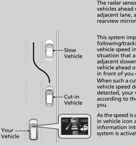
The radar sensor in the front grille detects vehicles ahead of you including those in the adjacent lane, and the camera behind the rearview mirror detects the lane markings.
