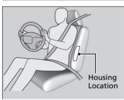
The side airbags are housed in the outside edge of the driver's and passenger's seat-backs.
