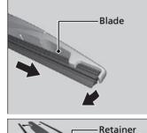
**3.** Slide the blade out of the wiper.
