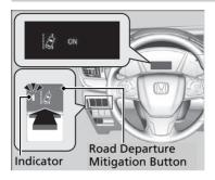
Press the Road Departure Mitigation button to turn the system on and off.
