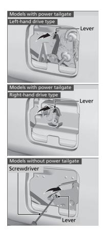
**2.** To open the tailgate, push the tailgate while pushing the lever to the right.
