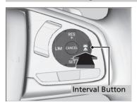
Press the 🖹 (interval) button to change the ACC with LSF following-interval. Each time you press the button, the following-interval (the interval behind a vehicle detected ahead of you) setting cycles through short, middle, long and extra long following-intervals.
