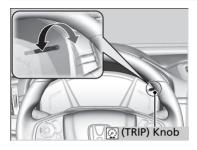
When the brightness of the meter is reduced, you can use the (2) (TRIP) knob to adjust instrument panel brightness. Brighten: Turn the knob to the right. Dim: Turn the knob to the left.
