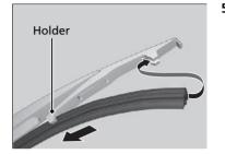
5. Slide the new wiper blade onto the holder.
