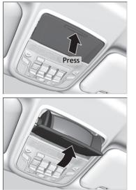
To open the sunglasses holder, press and release the indent. To close, press it again until it latches.
