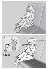
If a lap/shoulder seat belt cannot be used properly, position the child in a booster seat in the rear seat. For the child's safety, check that the child meets the booster seat manufacturer's recommendations.
