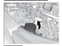
All models Pour the washer fluid carefully. Do not overflow the reservoir.
