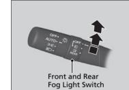
■ To turn the front fog lights on Rotate the switch up from the OFF position to the ‡ position. The ‡ indicator comes on.
