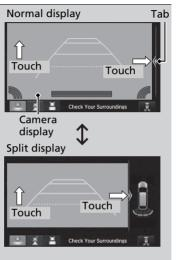
You can switch the display to normal display or split display by touching the tab vicinity or on the camera display.
